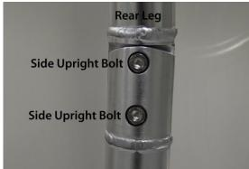
Attach Legs to Top Section at Estimated Width: This can be most easily done on the ground and will require four people to move the T-Top into the boat. Measure the approximate width of where you will install the T-Top over your center console. This does not need to be exact and will be adjusted when you move the T-Top to the boat. Be sure the legs are wide enough to fit around the console when placed in the boat as shown below.
