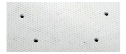
**Put 3M 5200 Adhesive in Holes and Base Location:** The 3M 5200 Marine Adhesive is a key structural part of any T-Top installation. Squirt 5200 into each hole and be sure it is filled with 5200. Then add a smooth layer about 1/16" thick between the four holes. The majority of the strength comes from the screws being bonded to the hole and the base being bonded to the deck adds additional strength. This should look like the image below.
