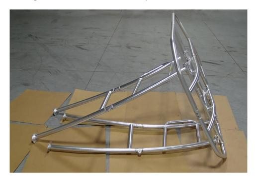
**Move the T-Top to the Boat**: It is easiest to have two people on the ground transfer the T-Top in the vertical position to two people in the boat. With only two people one can lift the canopy frame and the second can lift at the base of the legs to transfer to the boat in the
